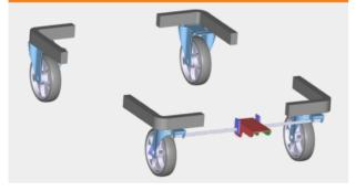
Two swivel castors are connected by a hexagonal rod. With one step on the lock release, both castors are locked or released again.
