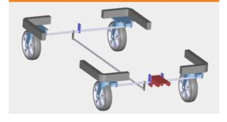
When 4 swivel castors are used, all the castors are connected to one another via carrier or control rods.
